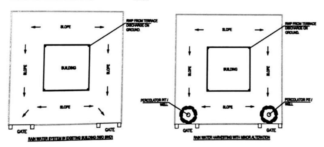
If, the existing premises have open storm water drain with gratings, then drill holes of 100 mm or 150 mm diameter at the bottom of the Storm Water Drain. This will allow water to percolate into the soft soil while flowing through the SWD. These are the easiest ways to introduce Rain Water Harvesting in existing premises with minimum expense. This will not only allow percolation of rain water into the ground but
